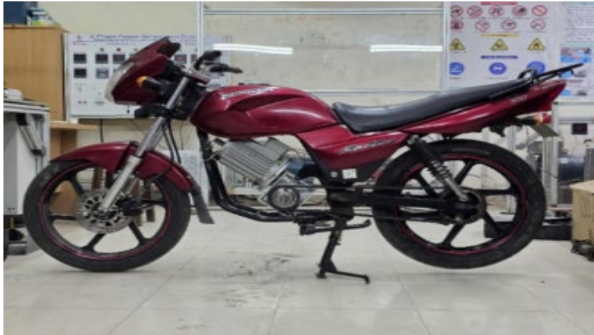
Figure 3. Conversion of a conventional motorcycle into an electric motorcycle at the IUB Formula E laboratory setup.
