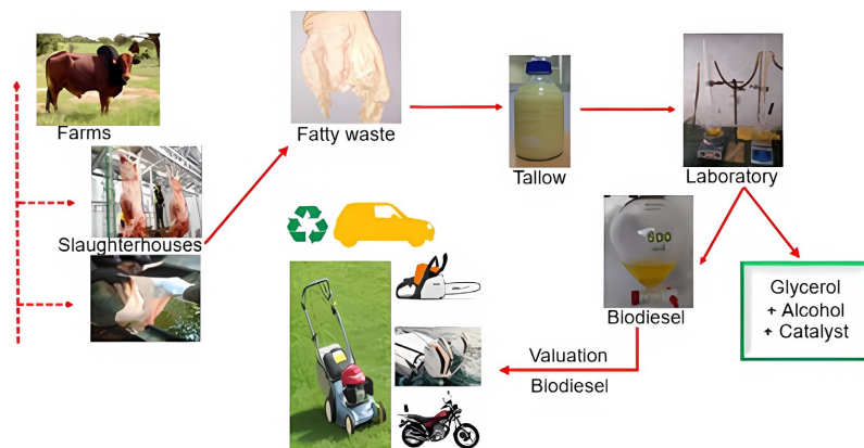
Figure 1. Overview of the process for recovering value from slaughterhouse fat residues.
