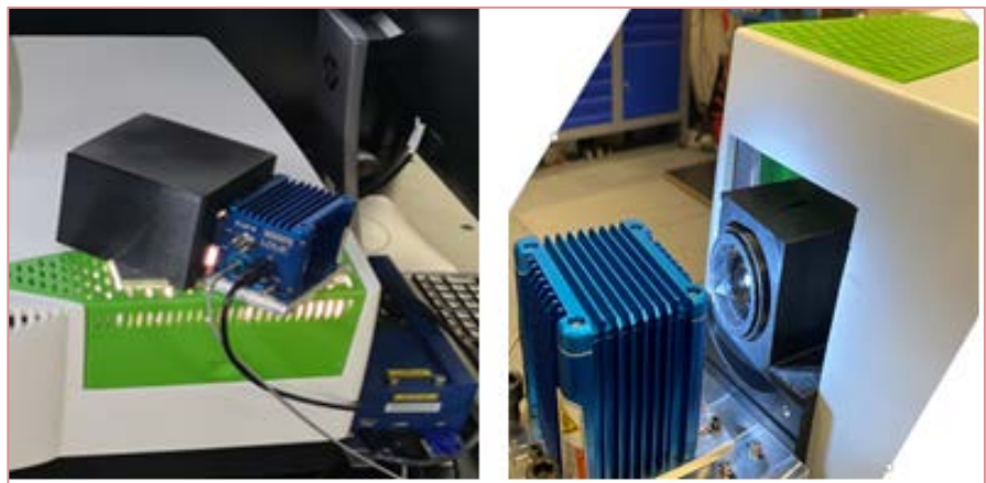
Figure 4. Changes were made to the spectrometer's radiation source.
