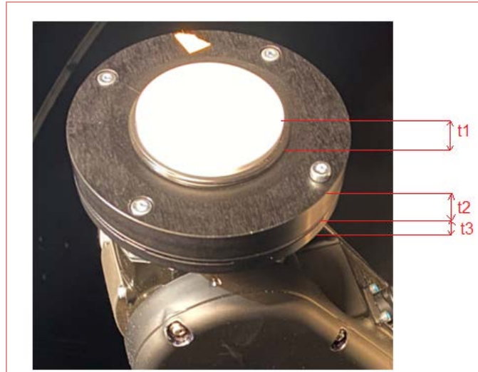
Figure 9. Shows measurements of the sample holder and the sample thickness of the robot arm.
