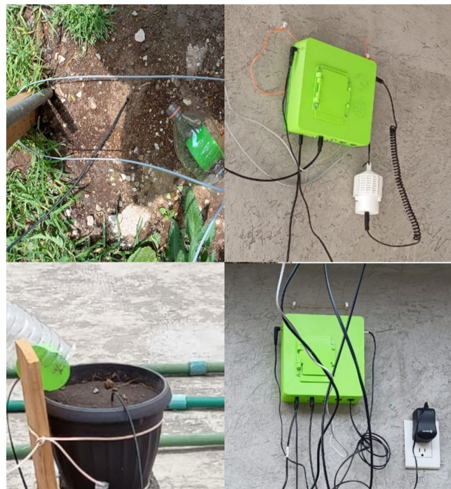
Figure 1. Experimental setup for surface and internal soil temperature measurements in field soil (top left) and potted soil (bottom left), from Experiment 1.
