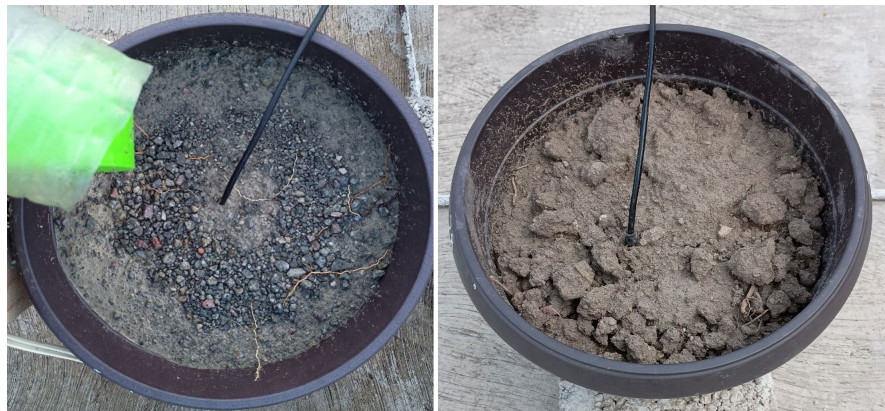
Figure 2. Setup for measuring surface and internal temperatures in pots filled with sand (left) and soil (right), as part of Experiment 2.
