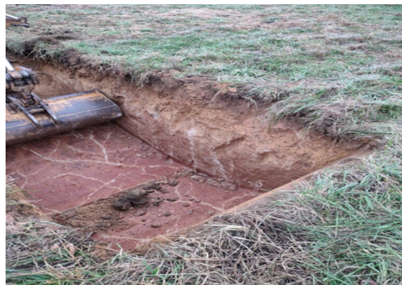
Figure 1. An exposed fragipan soil showing the inter-prismatic gray veins that separate the consolidated, impermeable prismatic matrix.
