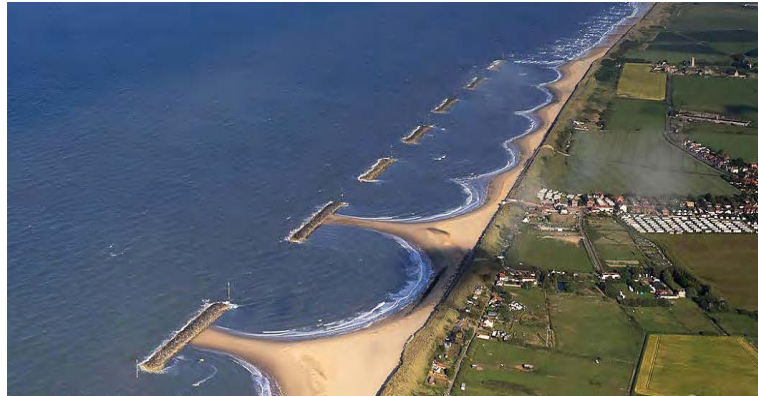
Figure 10. Breakwater battery: long-term solution [4].
