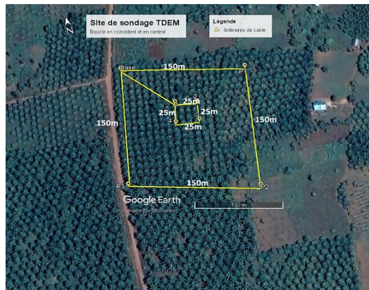
Figure 4. Configuration of a TDEM loop for a coincident survey with a 150 m loop.
