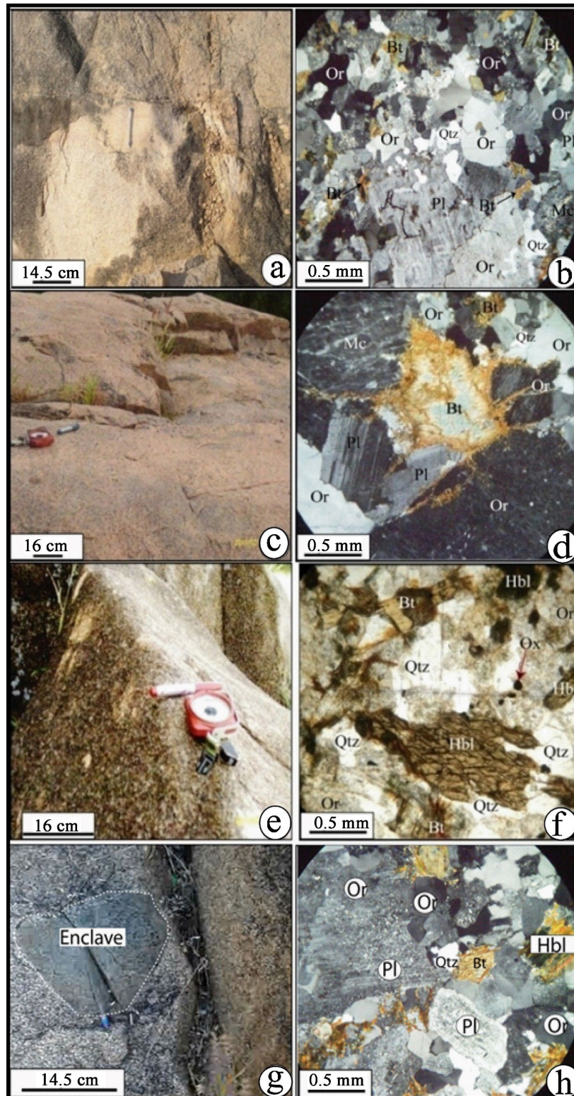
Figure 3. (a) Slab outcrop of pink granites from Mount Mouta; (b) Portion of thin section of pink granites. Note the coexistence of orthoclase and microcline crystals, (c) Slab outcrop of pink microgranites to the SW of Mount Gabra, note the presence of microfractures on the slab of pink microgranites; (d) Portion of thin section of biotite microgranites; (e) Block outcrop of syenite from Mount Doré; (f) Portion of thin section of syenite; (g) Enclave of granodiorites in the syenite from Mount Illi; (h) Portion of thin section of granodiorites.
