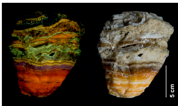
Figure 2. Photographs of silica sinter sample under normal light (right) and ultraviolet rays (365 nm) (left).
