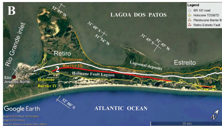
Figure 4. Simplified geological map for Bujuru (A) and Retiro (B) HM deposits. Lagoa do Peixe (1) and Retiro-Estreito (2) normal fault traces define the Northwest escarpment against Pleistocene sediments. Legend GPR radargrams: a) Figure 9 radargram; b) Figure 10 radargram; c) Figure 11 radargram. i-iii: boreholes locations in the Bujuru area.
