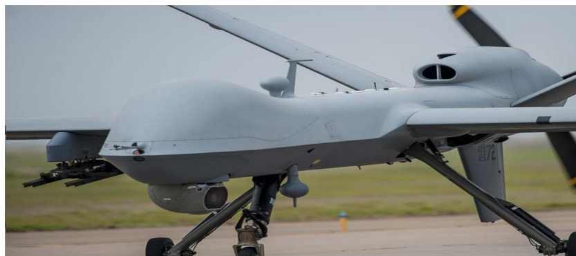
Figure 2. Heavy universal unmanned aerial vehicle UAV MQ-9 with sensor sensors installed on a stabilized sighting platform with a powerful zoom, laser and infrared thermal imager, all-weather SAR radar with a synthesized aperture for high-precision remote environmental sensing, which can be used to map radiation fields in the “atmosphere” system—the underlying surface of the earth.
