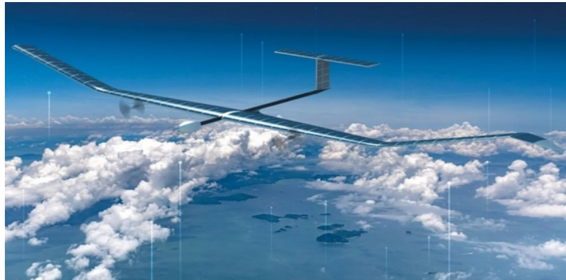
Figure 1. Zephyr S Airbus solar-powered high-altitude UAV pseudo-satellite suitable for remote environmental monitoring of natural and anthropogenic objects: wingspan—25 m, weight—about 75 kg, maximum flight altitude—up to 23,200 m, continuous flight duration—up to 3 months.
