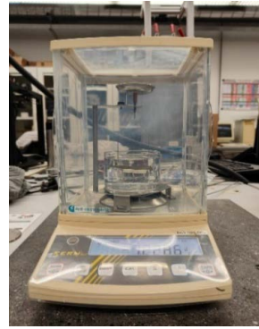
Figure 12. Density Archimedes' principle.
