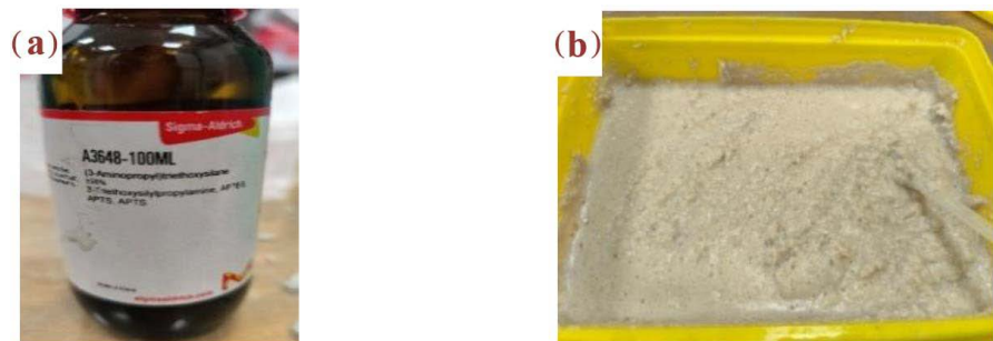
Figure 5. Silane treatment of chicken feather powder: (a) (3-aminopropyl) triethoxysilane (APTES), (b) APTES-treated feather powder.
