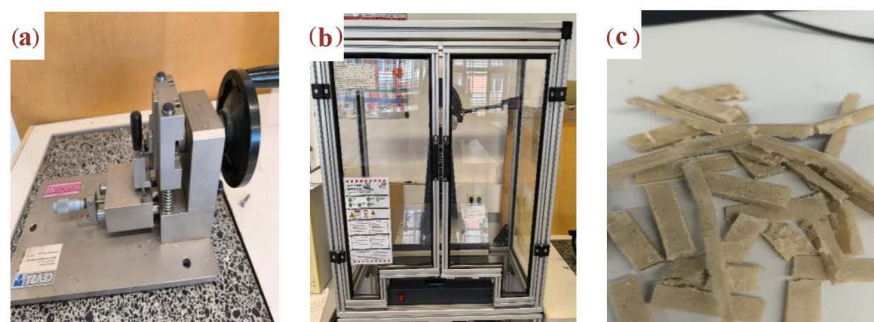
Figure 10. Impact testing: (a) Notch preparation machine, (b) Pendulum impact testing machine, (c) Fractured specimens after testing.
