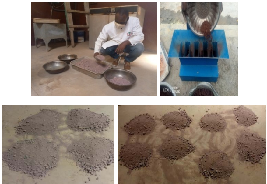
Figure 4. Preparation of material samples by quartering.
