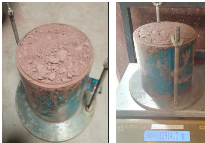
Figure 6. Measurement of the bulk density of 0/31.5 aggregate.
