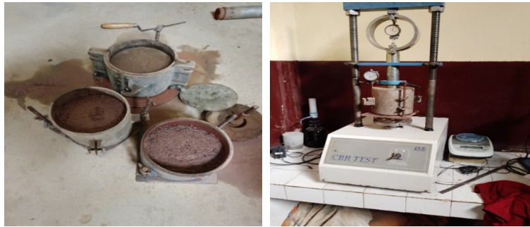
Figure 7. CBR test on 0/31.5 aggregate.
