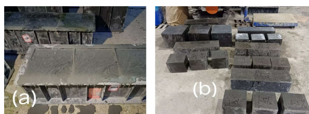
Figure 3. (a) fresh concrete cast specimen (b) spayed concrete specimens after demolding under 28 days curing process.
