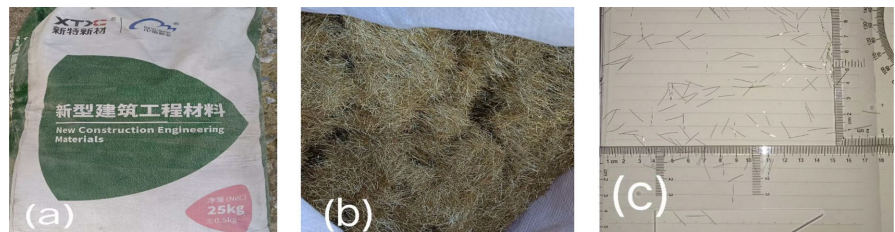
Figure 1. Materials used in the design mix: (a) ready-mixed UHPC reactive concrete powder, (b) 13 mm length UHPC steel fiber, and (c) measured steel fiber.
