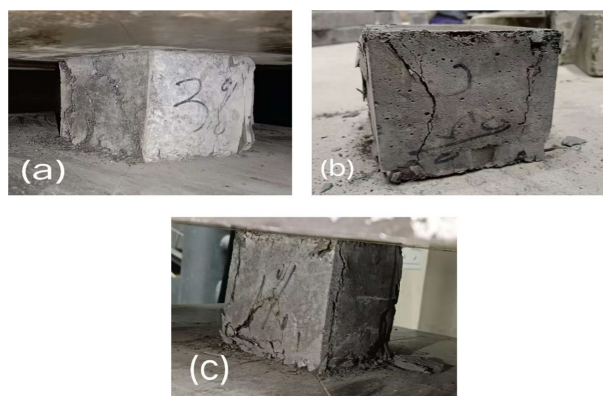
Figure 8. Failure mode after compressive failure for (a) 3%, (b) 2.5%, and (c) 1% steel fiber volume ratio.
