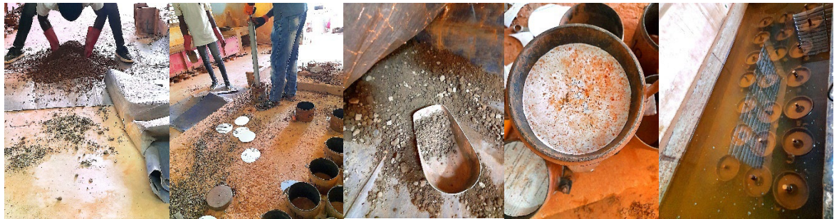
Figure 9. Principle of sample preparation for CBR test.
