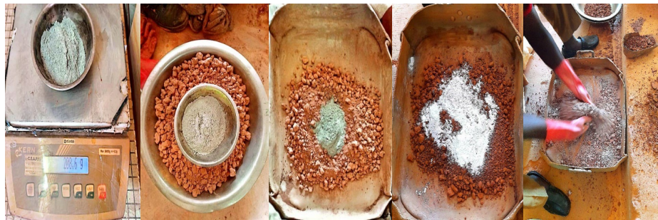
Figure 8. Principle of sample preparation for the Proctor test.
