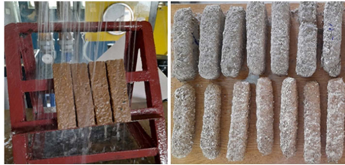
Figure 2. Test pieces in full erosion test and eroded test pieces.
