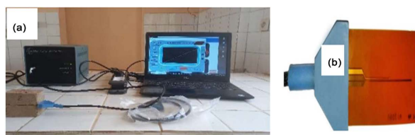
Figure 7. (a) FP2C device + computer, (b) Hot wire probe.
