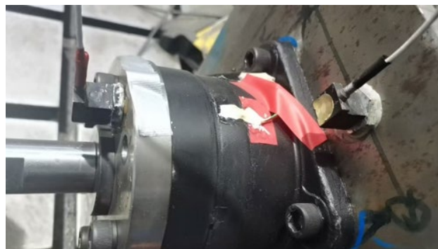
Figure 5. The attachment of strain gauges for strain measurement.
