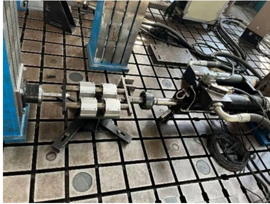
Figure 3. Uniaxial fatigue test rig for elastic support specimen.
