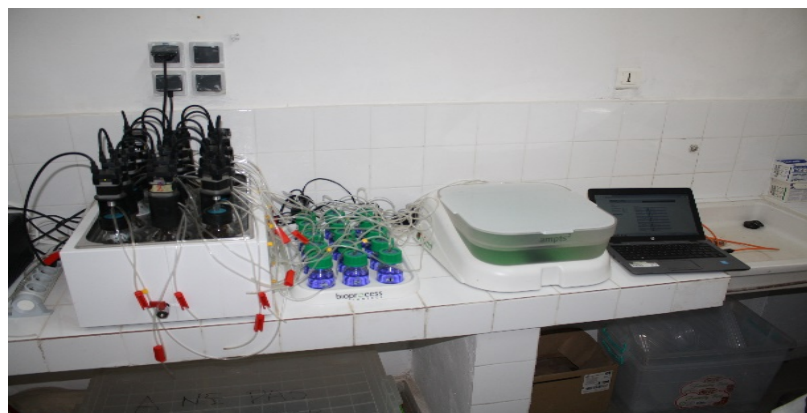
Figure 3. Photo of the AMPTS II (Automatic Methane Potential Test System II) methane potential analyzer device from Bioprocess Control deployed at LMI IESOL at the ISRA/IRD Bel Air center in Dakar, Senegal © J.-M. Médoc, April 2019.
