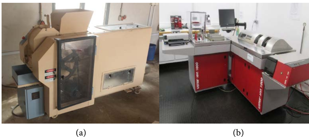
Figure 1. 10-saw gin (a) and integrated measuring chain (b) used for ginning seed cotton and analyzing the technological characteristics of the cotton fiber.
