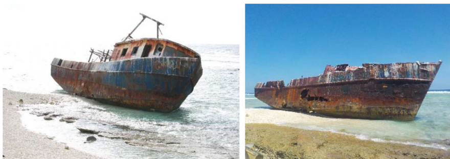
Figure 13. Degradation, between 2008 and 2015, of the tuna vessel Lily Mary, grounded in 2000, on the north-east coast of the atoll. Source: Tchekemian (2023).
