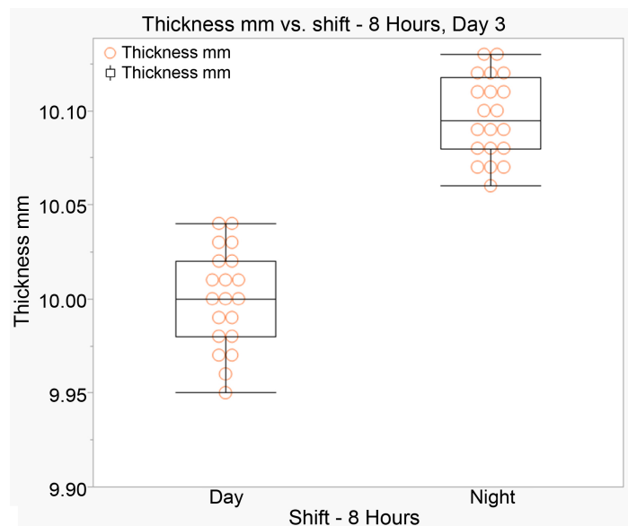
Figure 5. Box plot of ultrasonic thickness measurements for Day 3 comparing day and night shifts. Similar to the previous days, night shift measurements show a consistently higher distribution.
