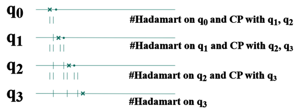
Figure 6. The structure of the QFT operation employed in this implementation is shown by the Inverse Quantum Fourier Transform Circuit.
