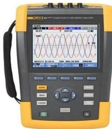
Figure 5. PQ data logger fluke 435.
