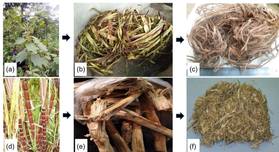
Figure 1. Some images of the fiber extraction process of the study. (a)—TC plant, (b)—TC bark, (c)—Extracted TC fibers, (d)—Sugar cane stalk, (e)—Bagasse, (f)—Extracted BS fibers.
