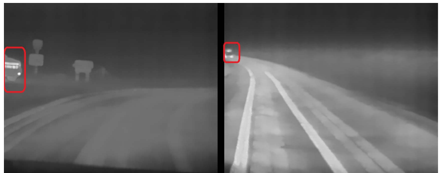
Figure 14. Images misclassified as not containing a trailing vehicle.
