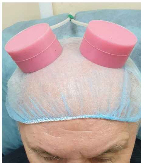
Figure 1. Location of piezoceramic sensors of mechanical microvibrations on the human head.
