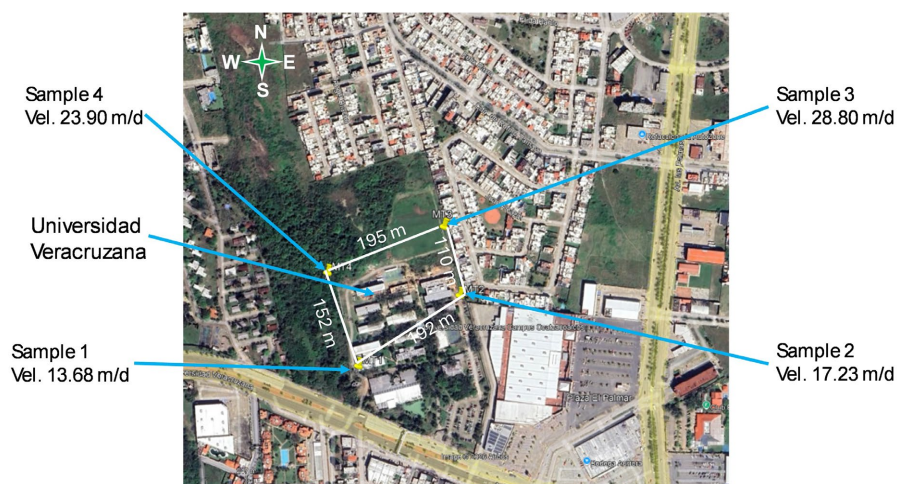
Figure 8. Location of samples S1 - S4 collected at the Universidad Veracruzana, Coatzacoalcos Campus. The four sampling points are close to one another; however, the apparent groundwater flow velocities differed at each one (13.68, 17.23, 28.80, and 23.90 m/d).
