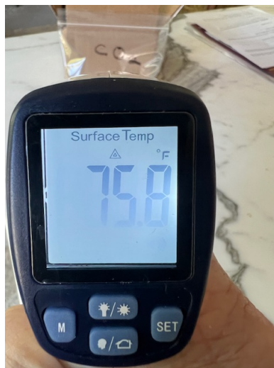
Figure 5. The temperature of the CO 2 bag taken after being exposed to the microwave oven.
