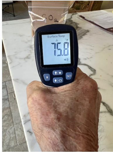
Figure 4. The temperature of the bag containing CO 2 taken before being exposed to the microwave oven.
