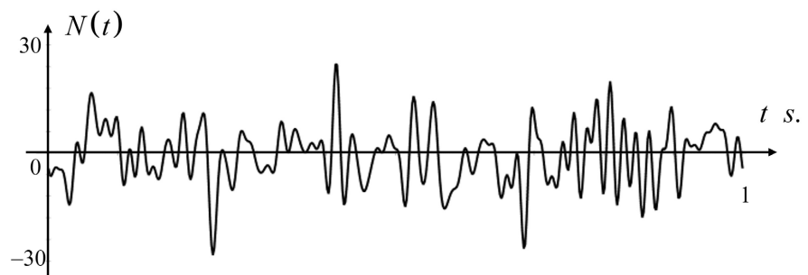
Figure 3. Analog representation of the noise realization obtained by the T-method at K=1 .
