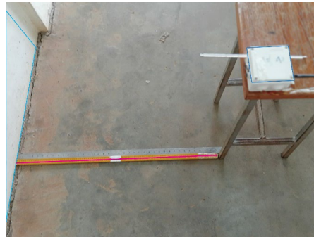
Figure 5. Ultrasonic sensor distance range testing against a wall obstacle measurement for sensor performance over distances of 100 cm, 200 cm and 300 cm.
