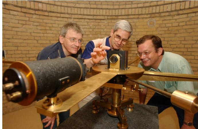
Figure 6. Reconstruction of the original Michelson interferometer located in the Michelson basement. Today the use of this Michelson interferometer is demonstrated by Dierk-Ekkehard Liebscher (center of the photo) to visitors of the Astrophysical Observatory Potsdam.
