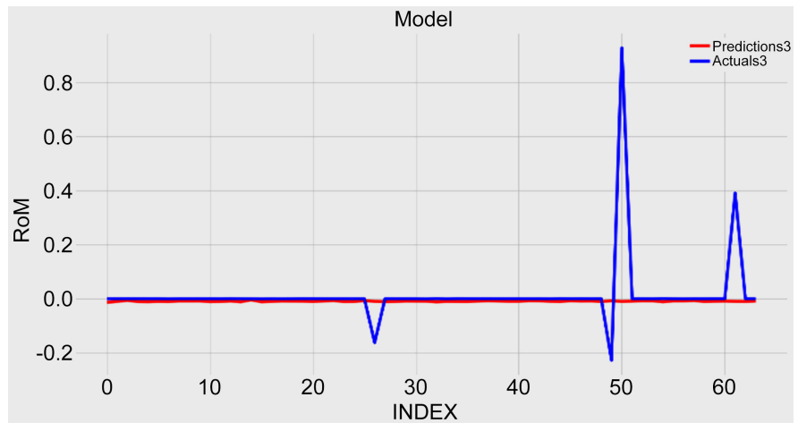
Figure 11. Line chart of actual and predicted rate of displacement using C-LSTM.
