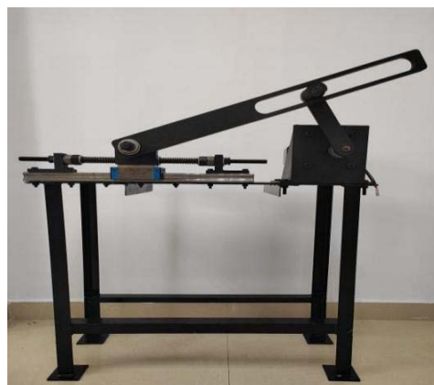
Figure 2. Experimental platform for dynamic performance of metamorphic mechanism for the groove pin pair with clearance.
